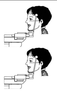
② Adjust the beam height so that the beam hits the patient's miniscule of the ear (hole). Then adjust the patient's head as to beam indicates Frankfort Plane (from miniscule of the ear to bottom of the eye orbit)
