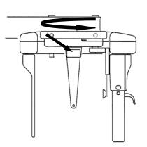
Rotate Ear Rod by holding the fixing portion of Ear Rod, align Ear Rod to exposure direction of Cephalo Front.
