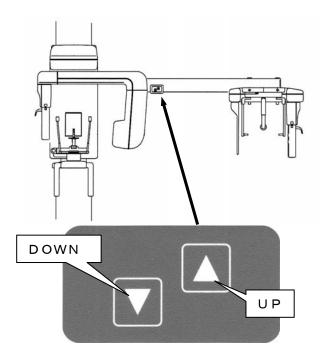
\* Push either of UP or DOWN key of Cephalo ARM Up-Down Panel, and move Sliding Unit up and down to align position of Ear Rod to near of external auditory foramen.
