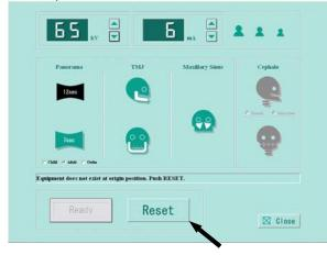
f you receive the message [Equipment is not at the original position. Push the RESET button.] Then click the [RESET button].
