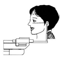
③Adjust the beam height so that the beam hits the patient's miniscule of the ear (hole). Then adjust the patient's head as to beam indicates Frankfort Plane (from miniscule of the ear to bottom of the eye orbit)
