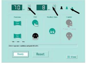
Setting kV Click kV  $\blacktriangle$  (UP)  $\cdot$  or  $\blacktriangledown$  (DOWN) to set kV.
