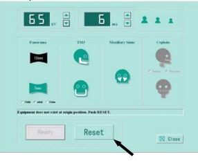
If you receive the message  $\lceil$ Equipment is not at the original position. Push the RESET button.] Then click the  $\lceil$ RESET button].
