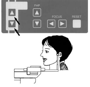
Depress either  $\bigcup P$  D O W N key on the Beam Control Panel or the one on the Sliding Unit to move position of Ear Rod(TMJ Frontal).
