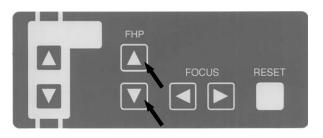
④ Depress either UP • DOWN key of Frankfort Beam on Beam Operation Panel and align Frankfort Beam Line with Frankfort Plane of a patient.
