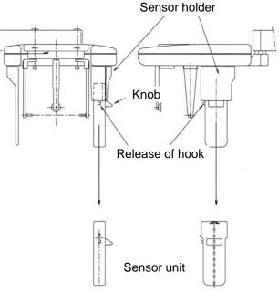
② Attach CCD sensor to Panorama Refer to 1 1. Operation Procedure for Panorama and 1. Preparation for exposure.
