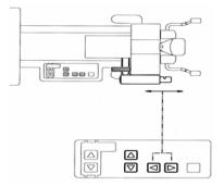
\* Forward and backward movement of the Focus Beam Line.
