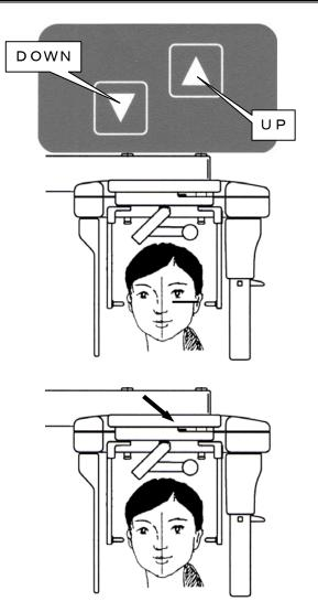
①Push either of UP or DOWN key ofU p and down Movement Panel on CephaloAR M to insert ear rod into external auditoryfora men of a patient with fine adjustment.
