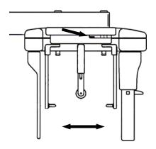
②Move Open-Close Lever for Ear Rod of Cephalo stat to open Ear Rod maximally.
