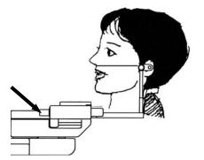
③Rotate the knob of the Chinrest ASSY to insert Ear Rod (TMJ Frontal) into auricular holes of a patient and fix Ear Rod lightly.
