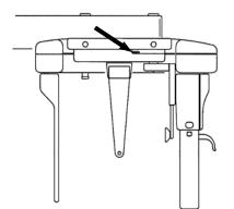
②Move Open-Close Lever for Ear Rod of Cephalo stat to open Ear Rod maximally.
