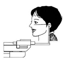
② Adjust the beam height so that the beam hits the patient's miniscule of the ear (hole). Then adjust the patient's head as to beam indicates Frankfort Plane (from miniscule of the ear to bottom of the eye orbit)
