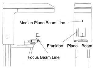
②"Median Beam Line", "Focus Beam Line", and "Frankfort Plane Beam Line" are equipped
