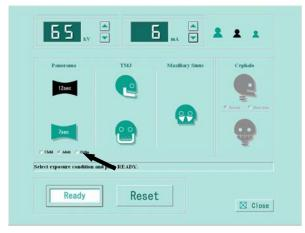
Click Child or adult or ortho (Ortho radial exposure). \* Ortho : Radiography of less tooth overlap.
