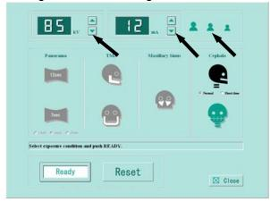
Set kV Click kV  $\blacktriangle$  (UP)  $\cdot$  or  $\blacktriangledown$  (DOWN) to set kV. Set mA Click mA  $\blacktriangle$  (UP)  $\cdot$  or  $\blacktriangledown$  (DOWN) to set mA.
