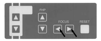
1 Depress either Forward Movement • or Backward Movement key of FOCUS switch on the Beam Operation Panel to turn Patient Positioning Beams on.
