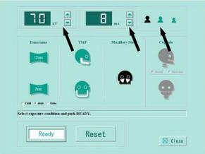
Setting kV Click kV  $\blacktriangle$  (UP)  $\cdot$  or  $\checkmark$  (DOWN) to set kV. Click mA  $\blacktriangle$  (UP)  $\cdot$  or  $\checkmark$  (DOWN) to set mA.
