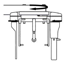
(T)Rotate Ear Rod by holding the fixing portion of Ear Rod, align Ear Rod to exposure direction of Cephalo Lateral.
