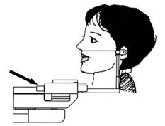
④Rotate the knob of the Chinrest ASSY to insert Ear Rods (TMJ Lateral) into auricular holes of a patient and fix Ear Rod.
