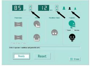
Setting kV Click and select right side of kV  $\blacktriangle$  (UP) • or  $\blacktriangledown$  (DOWN). Setting mA Click and select right side of mA  $\blacktriangle$  (UP) • or  $\blacktriangledown$  (DOWN). Or click upper right patient display. In this case, depend on patient, adjustment of kV • mA will be necessary
