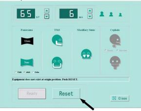
If you receive the message [Equipment is not at the original position. Push the RESET button.] Then click the [RESET button].
