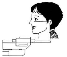
④ Rotate the knob of the Chinrest ASSY to insert Ear Rods (TMJ Lateral) into auricular holes of a patient and fix Ear Rod.
