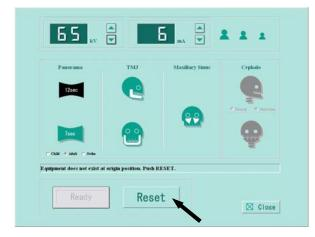
f you receive the message 「Equipment is not at the original position. Push the RESET button.」 Then click the 「RESET button」.
