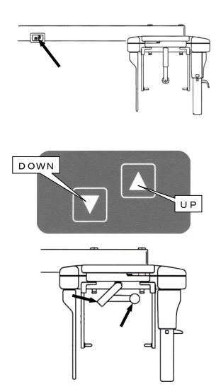
①Push either of UP or DOWN key of Cephalo ARM Up-Down Panel, and move Sliding Unit up and down to align position of Ear Rod to near of external auditory foramen.
