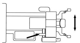
③ Rotate the knob of Chinrest Unit to open Head Holding Rods maximally.
