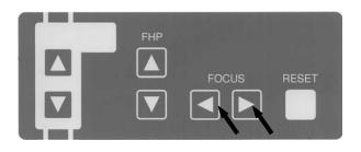
⑥Depress either Forward Movement • or Backward Movement key of FOCUS Beam switch on the Beam Operation Panel, and align Focus Beam Line with roots of upper and lower anterior teeth.
