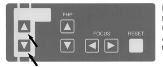
Depress either UP DOWN key on the Beam Control Panel or the one on the Sliding Unit to move position of Ear Rods(TMJ Lateral). Align ear rods to patient's external auditory foramen.
