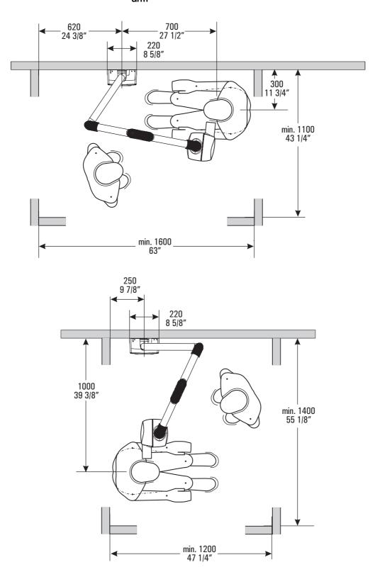
Minimum dimensions for X-ray rooms with 410 mm (16 1/8") support arm
