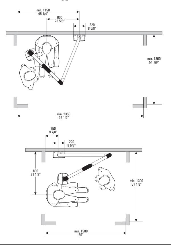
Minimum dimensions for X-ray rooms with 950 mm (37 3/8") support arm
