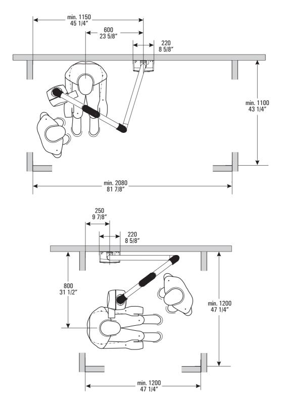
Minimum dimensions for X-ray rooms with 700 mm (27 1/2") support arm
