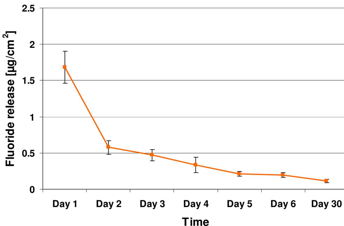
Fig. 8: Fluoride release of Helioseal F over 30 days [25]
