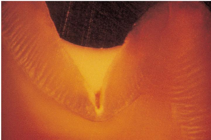
**Fig. 5: The sealant forms a smooth hygienic surface. If the sealing is tight, the microorganisms are cut off from the supply of substrates and are no longer viable.**
