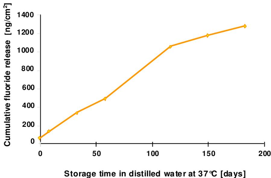
Fig. 9: Cumulative fluoride release of Helioseal F; mean value of 20 specimens [27].
