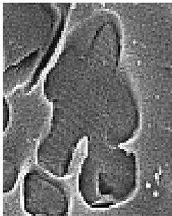
Fig. 6: Middle section of Fig. 5 (magnified) The striation in the dissolved areas shows the lamellar structure of leucite crystals – a result of dendritic growth.
