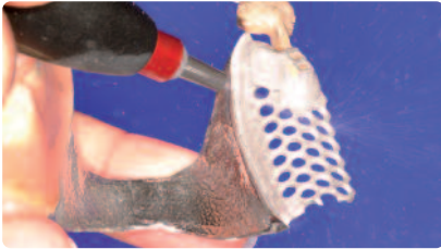
Blast with Type 100 \text{Al}_2\text{O}_3 at 2-4 bar / 29-58 psi pressure.
