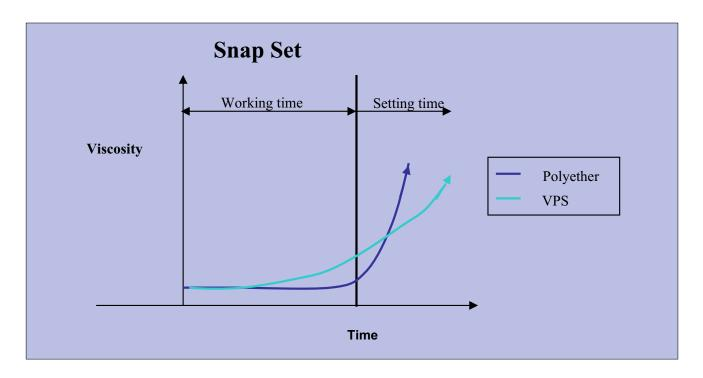
The brief transition between working time and setting, which is typical for polyether, is referred to as Snap Set.
