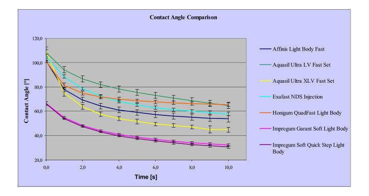
During the working time at 45 seconds after start of mixing, a drop of water was placed on the impression material, and the contact angle of the drop was measured. The data is shown in one second increments.
