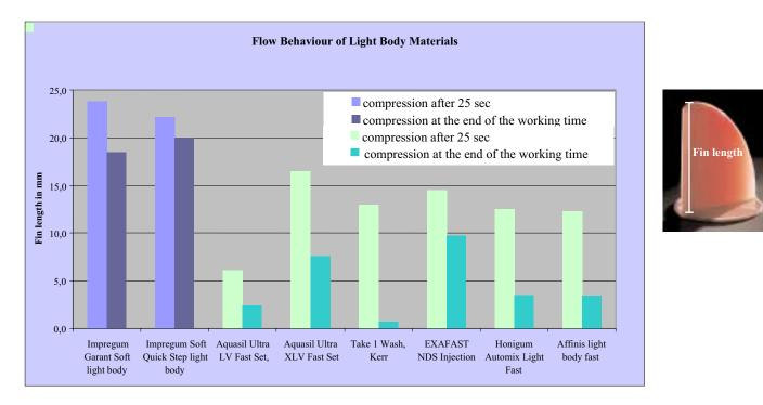
Both polyether impression materials exhibit significantly better flow properties than the VPS materials, at the beginning as well as at the end of the working time. It is also important to note that the flow properties of the polyether materials remain comparatively throughout the working period.
