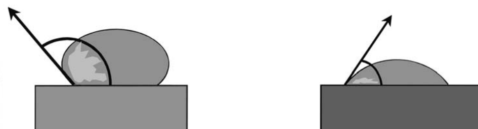
Fig. 12: A water droplet on a hydrophobic surface shows a contact angle of more than 90°; on a hydrophilic surface, however, the contact angle is less than 90°
