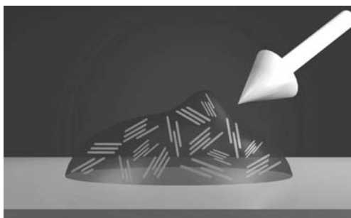
Fig. 8: Due to the crystallisation effect, triglycerides in the polyether form a three-dimensional lattice which lends the polyether a high level of viscosity
