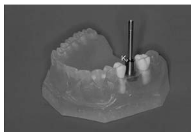
Fig. 17: Upper Jaw Model: original test specimens fitted in the upper jaw model. The mounting post is pointing towards occlusal; a notch (K) marks the mesial position.
