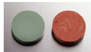
Fig. 6b: Superior mixing quality of Imprint™ 3 Penta™ Putty with the Pentamix™ Mixing Unit (left) compared with a putty mixed by hand (right, Express™ STD Putty).
