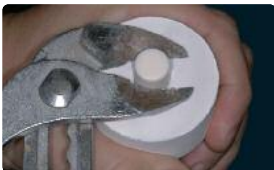
The Alox plunger is already very clean if it is removed with tongs from the investment material. Check the cleanness and blast with \text{Al}_2\text{O}_3 if required.
