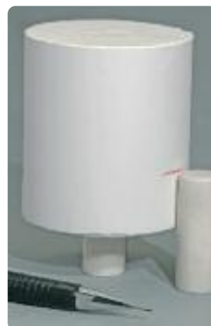
Mark the length of the Alox plunger.
