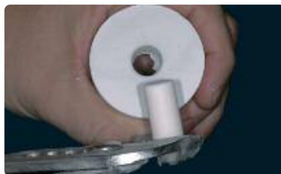
The Alox plunger is already very clean if it is removed with tongs from the investment material. Check the cleanness and blast with \text{Al}_2\text{O}_3 if required.
