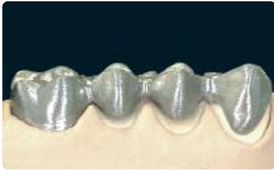
Surface finishing before blasting
