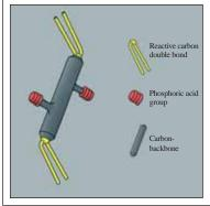
Acidic methacrylate monomers contain **phosphoric acid groups** and **reactive carbon double bonds** which are connected with each other via a carbon backbone.
