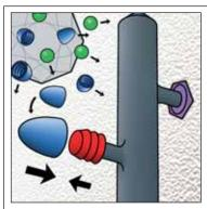
The remaining phosphoric acid groups of the methacrylate monomers are **neutralized** by ions, which are released from the **fillers** during the setting reactions.
