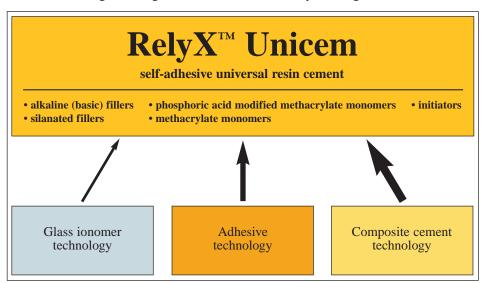
strength comparable to that of adhesive resin systems demanded new monomers, fillers, and initiators. Now, based on the same reliable and proven chemistry, the formulation of the capsule system was transformed into a paste/paste system for the Clicker™ Dispenser application.
