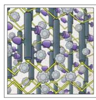
The methacrylate monomers and fillers are firmly linked and permanently embedded in the three-dimensional network of the cement matrix.
