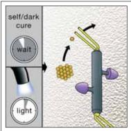
Simultaneously, setting of the cement takes place through the **radical polymerization reaction** of the methacrylate monomers.
