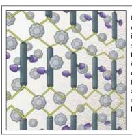
RelyX™ Unicem cement is cured by the radical polymerization reaction. Thus, successively a highly cross-linked three-dimensional network is formed consisting of methacrylate molecules and fillers. During this process the cement matrix changes from an initially hydrophilic to a hydrophobic condition.
